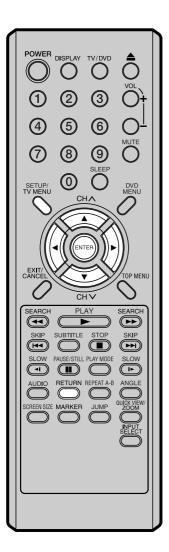
1 Press SETUP/TV MENU in the stop mode. Press ◀ or ▶ to select option, then press **v** or ENTER. ◄►/Enter/Setup/Return 2 Press ▲ or ▼ to select "Select Fih Files". ()TV Screen 4:3 🗖 Display Picture Mode On Auto JPEG Interval Off Select Files
